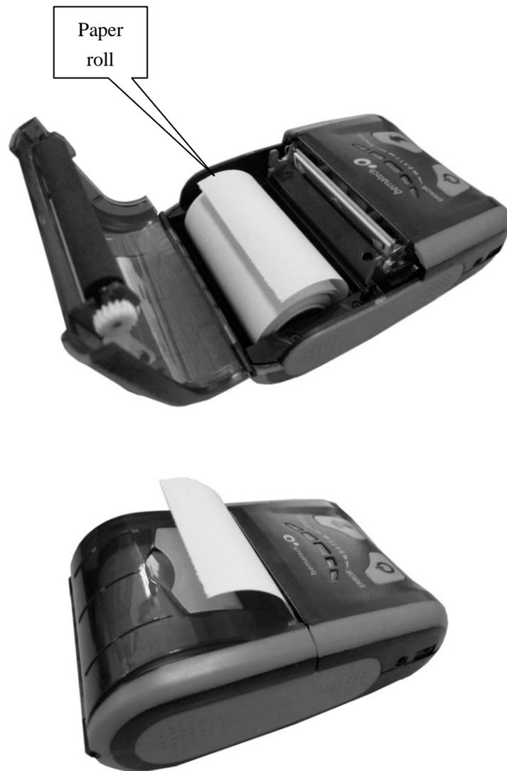
1. Pull up the cover level or press on both sides of cover to open it.
